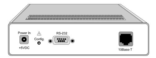
Figure 3-13: Ethernet LanProbe Rear Panel
